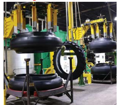
Titan has invested $2 million in its Iowa tire plant. The investment includes the addition of two 104-inch curing tire presses.
