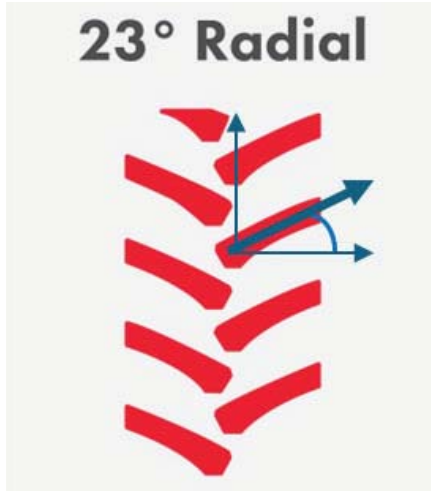
A 23-degree lug angle is usually flatter, while the 45-degree lug has more of a vertical point, according to Chris Neidert of Yokohama TWS.
