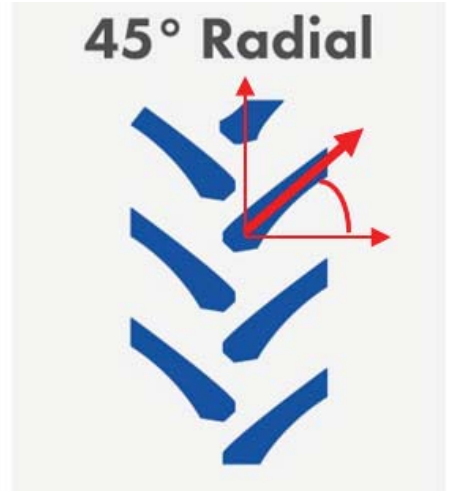
A 23-degree lug angle is usually flatter, while the 45-degree lug has more of a vertical point, according to Chris Neidert of Yokohama TWS.
